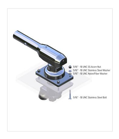
We recommend using nylon/fiber washers, stainless steel washers, and stainless steel acorn nuts to complete the mounting arrangement. Clean up excess sealant with acetone if necessary (DO NOT USE alcohol-based cleaners).
