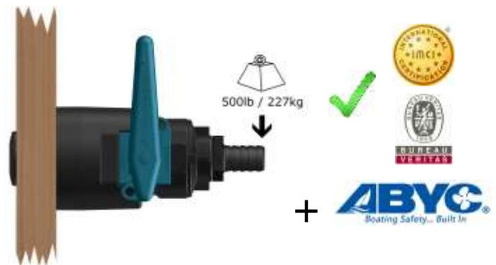
TruDesign Skin Fittings (Thru Hulls), when assembled together with TruDesign Ball Valves and Load Bearing Collars, comply with ABYC H-27 standards. This allows the entire assembly to withstand a 500lb (226.8kg) load applied to the inboard end of the assembly (i.e. from the Ball Valve's Tail fitting) for a minimum of 30 seconds without any damage occurring
